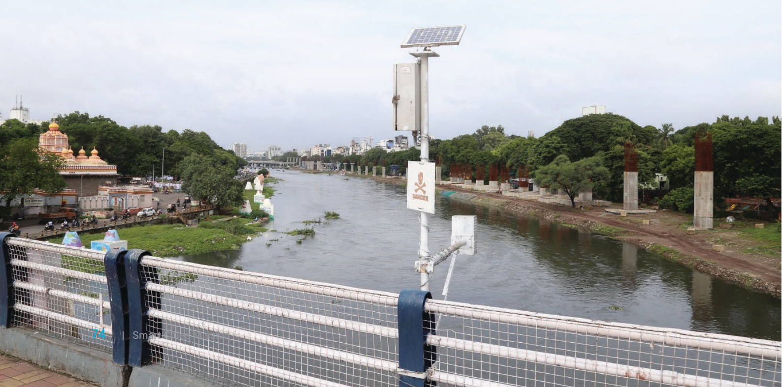
Image 33: Pune Smart City has installed more than 50 flood sensors at strategic locations as part of an integrated approach to disaster risk management. Source: Pune Smart City
