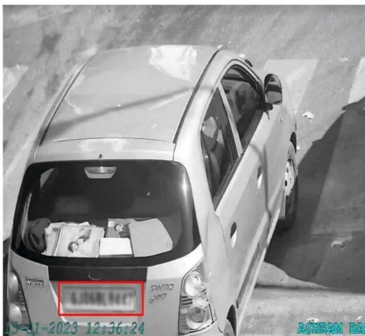
Image 43: Ahmedabad Smart City has installed 2,142 Automatic Number Plate Recognition (ANPR) cameras at traffic junctions which feed real-time data to ICCC, enabling effective monitoring of traffic violations. The intervention has led to improved revenue collection from fines for traffic violation. Source: Ahmedabad Smart City.
