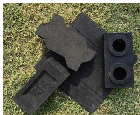
Figure 1 Silica Plastic Waste Blocks
